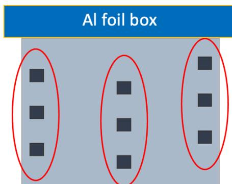
Figure 2: Schematic of subsample locations from a roll of Al foil.
