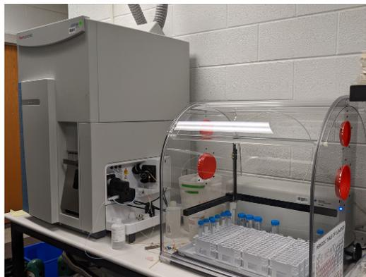
Figure 1: ICP-MS and autosampler used for analysis of digested Al samples.
