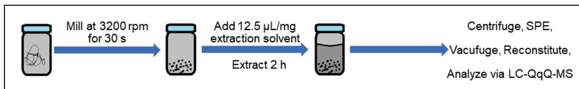
**Figure 3.** Schematic of extraction methods comparison procedure
