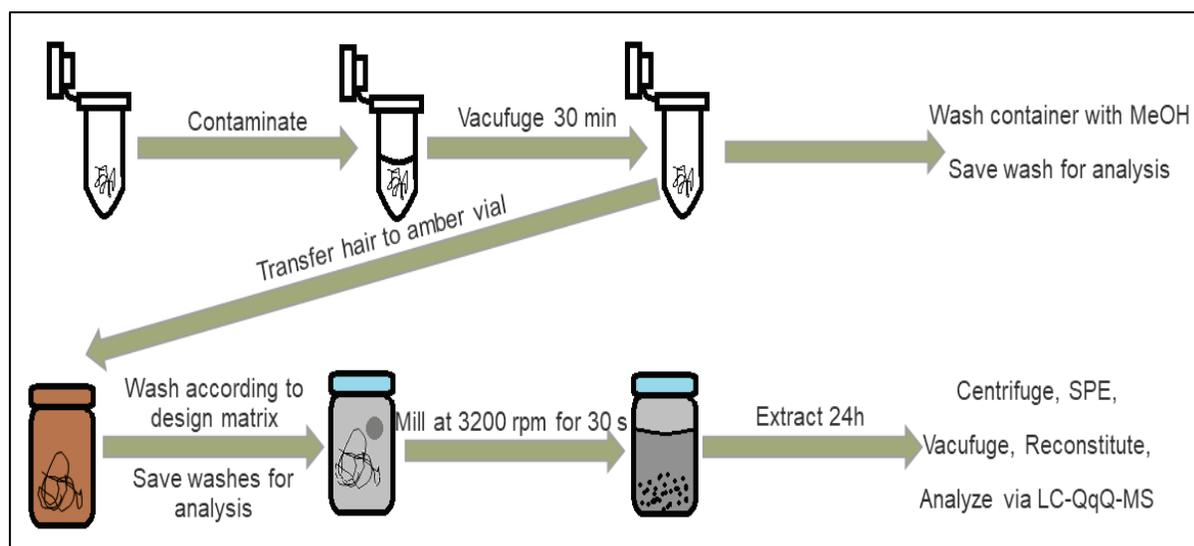
**Figure 1.** Schematic of decontamination DoE procedure.
