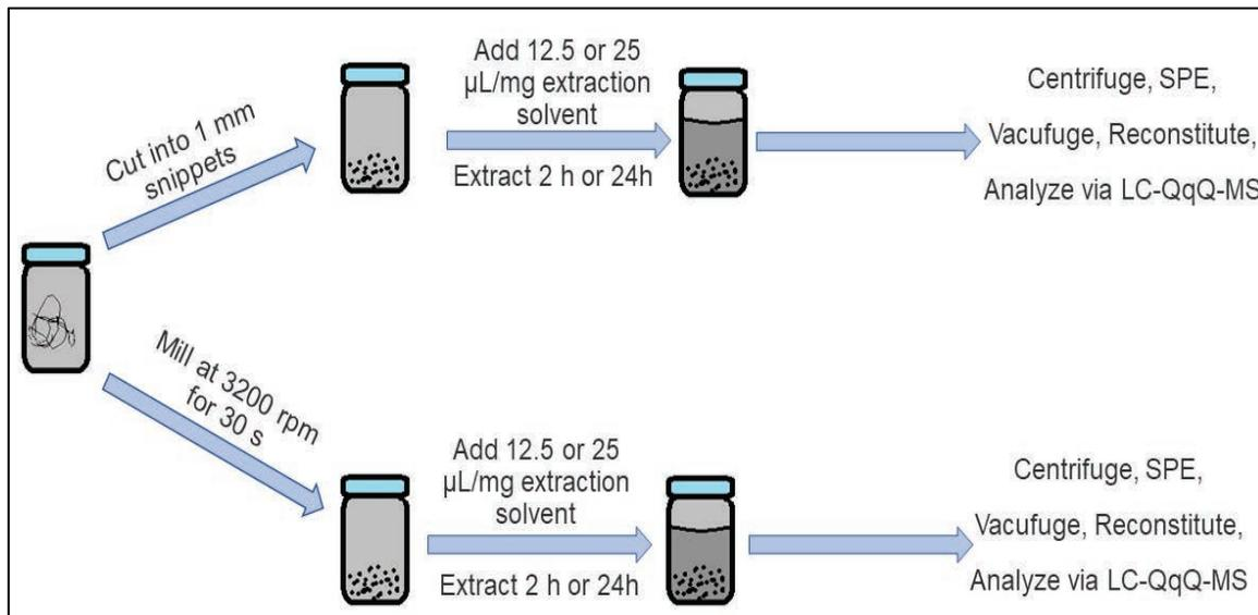
**Figure 2.** Schematic of pretreatment DoE procedure.
